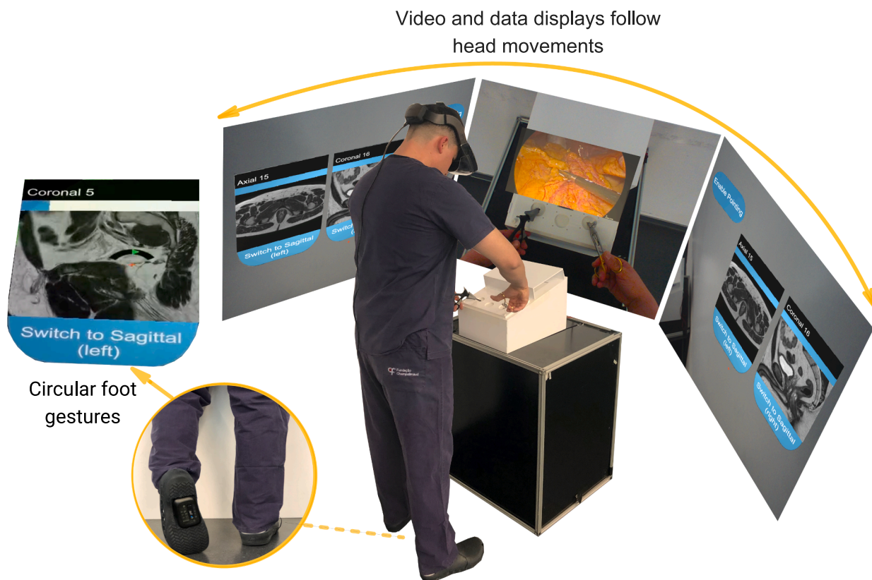
Fig. 5. A conceptual sketch of how the video and the data are displayed. Because the video follows head movements, looking to the side to visualise patient data would hide it. To implement foot movement detection, a mouse was introduced inside the rubber clogs used by the surgeons.
