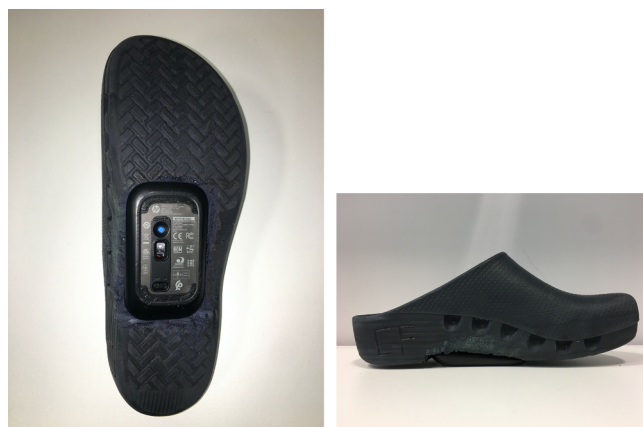
Fig. 4. Mouse clog. We can observe the wireless mouse does not interfere with the clog form factor.
