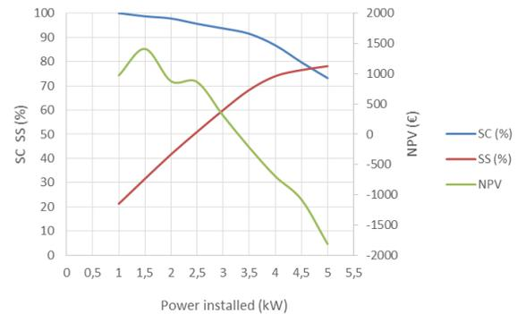
Figure 9. Evolution of  $NPV$ ,  $SC$  and  $SS$  with storage from  $2kW$  of power installed
