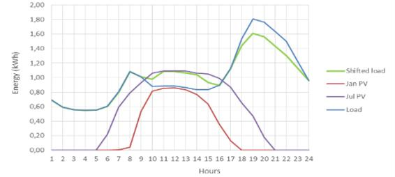
Figure 5. Limited load shifting allows less than 20% power increase
