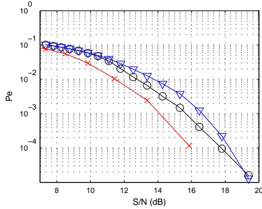
Figure 10: Probability ( $P_e$ ) of error versus SNR for algorithm II for 16-QAM modulation.  $\circ$  is with impulsive noise reduction;  $\nabla$  is without impulsive noise reduction and  $\times$  is the Zhidkov algorithm.
