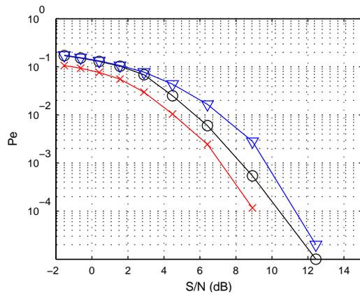
Figure 9: Probability ( $P_e$ ) of error versus SNR for algorithm II for QPSK modulation.  $\circ$  is with impulsive noise reduction;  $\nabla$  is without impulsive noise reduction and  $\times$  is the Zhidkov algorithm.
