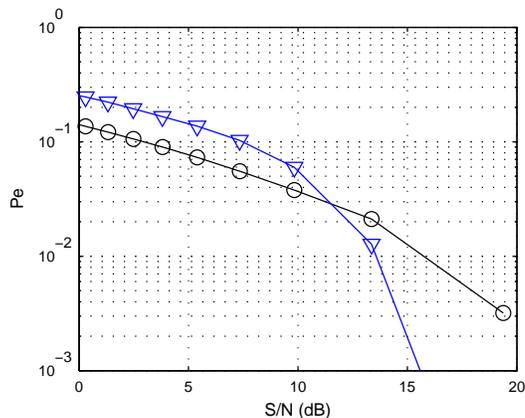
Figure 12: Probability ( $P_e$ ) of error versus SNR for technique III for 16-QAM modulation.  $\circ$  is with impulsive noise reduction and  $\nabla$  is without impulsive noise reduction.
