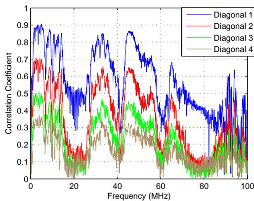
Figure 3: Values for Correlation coefficient of adjacent OFDM carriers, with a distance of one (diagonal 1), carriers with a distance of two (diagonal 2), three and four. The values are taken from the corresponding diagonal of the correlation coefficient matrix. The correlation decreases with increasing distance. The length of the OFDM symbols was 2467 samples at 200 MHz.
