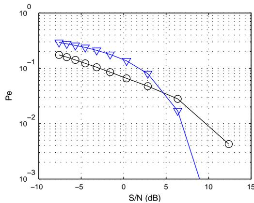
Figure 11: Probability ( $P_e$ ) of error versus SNR for technique III for QPSK modulation.  $\circ$  is with impulsive noise reduction and  $\nabla$  is without impulsive noise reduction.
