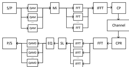
Figure 6: OFDM MODEM block structure with an equivalent shorter time duration of the OFDM symbol.
