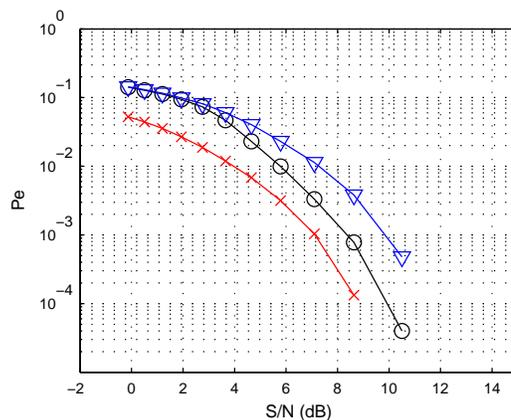
Figure 7: Probability ( $P_e$ ) of error versus SNR for algorithm I for QPSK modulation.  $\circ$  is with impulsive noise reduction;  $\nabla$  is without impulsive noise reduction and  $\times$  is the Zhidkov algorithm.
