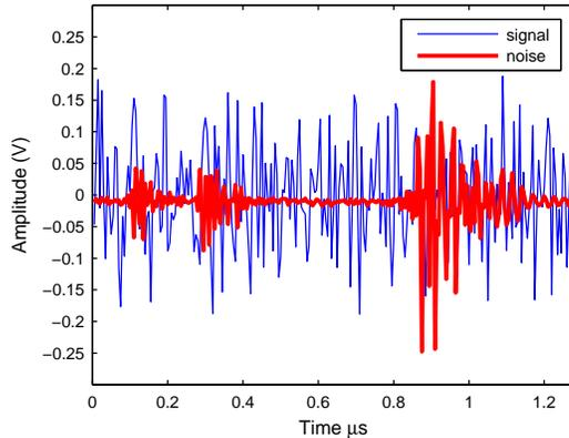
Figure 2: Plot of typical signal (in blue) and noise (in red) for a SNR of 7 dB and for the duration of one typical OFDM symbol. Sampling rate was 200 MHz.
