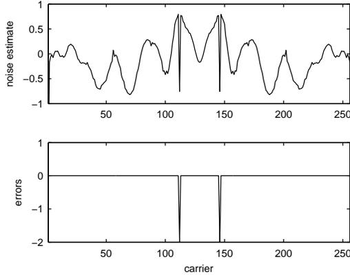
Figure 4: The noise estimate and the demodulation errors. It can be seen that the noise signal is smooth with two abrupt changes corresponding to the demodulation errors.
