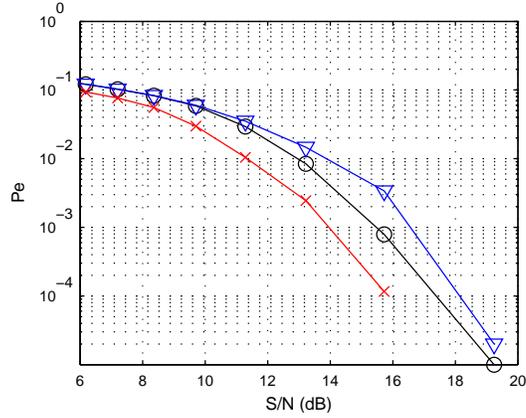
Figure 8: Probability ( $P_e$ ) of error versus SNR for algorithm I for 16-QAM modulation.  $\circ$  is with impulsive noise reduction;  $\nabla$  is without impulsive noise reduction and  $\times$  is the Zhidkov algorithm.
