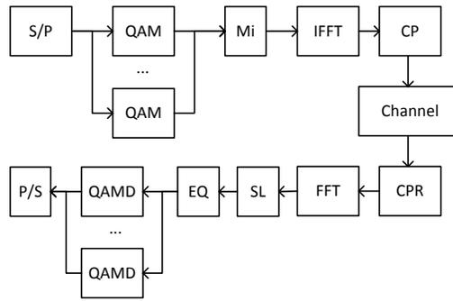
Figure 1: OFDM MODEM.
